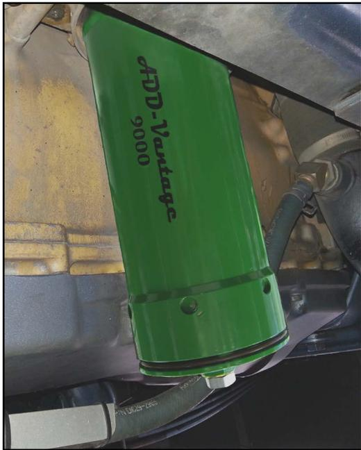
One Eye Industries ADD-Vantage 9000 Magnetic Filter easily fits traditional filter mounts.
