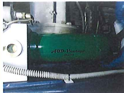
Magnetic technology replaces the HC35 Filter on a V47 wind turbine
