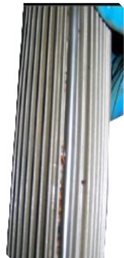
CONTAMINANTS CAPTURED BY THE STAINLESS-STEEL CLOTH ELEMENT
