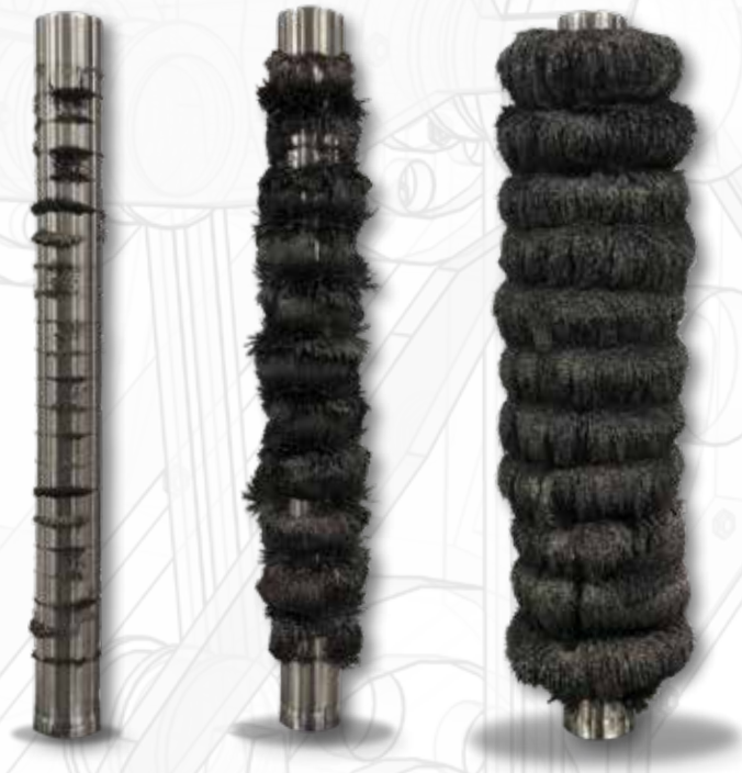
1" magnetic filter elements with varying loads of contamination
